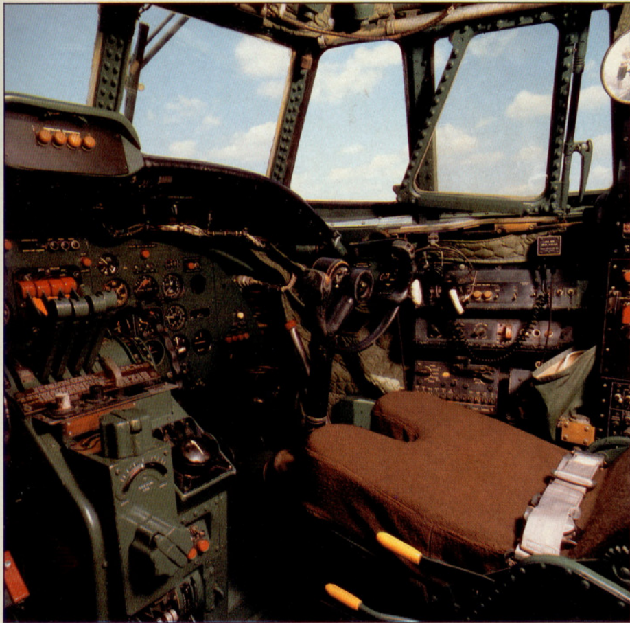
The view from the captain's seat (left). The pilots have little beyond throttles, tachs, and MP gauges in the way of engine controls and instruments; those were reserved for the flight engineer (above), who was always a certified mechanic. The FE, the busiest man in the cockpit, was flanked by additional controls and indicators not visible here.
